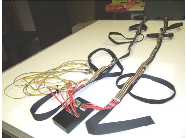
Figure 5. The 30-accelerometer module with the harness and all sensors attached: eight accelerometers are distributed over each leg, close to the joints; the other 14 sensors are situated on the upper body and arms.
