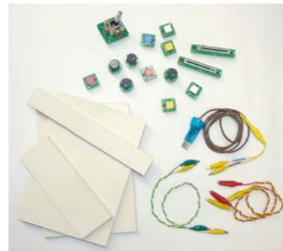
Figure 3. The VGK components: Substrate fabric, VoodooPin controls, and cable interconnects.
