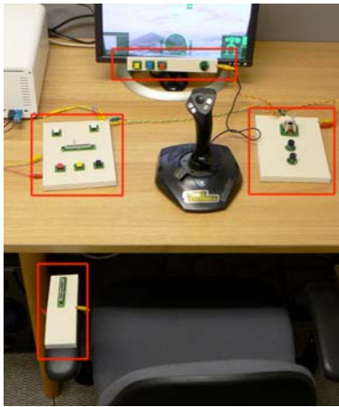
Figure 4. The completed ‘mech cockpit’ with four control substrates: Lower monitor bezel, desk (right and left of the joystick) and left chair armrest.
